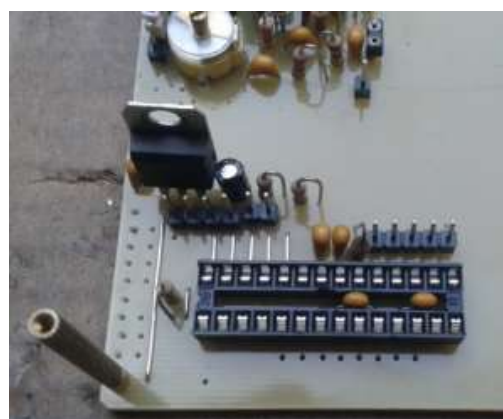
Microcontroller section (assembled) of the DDS VFO for 14+ MHz "Walki-Talkie" SSB Transceiver
