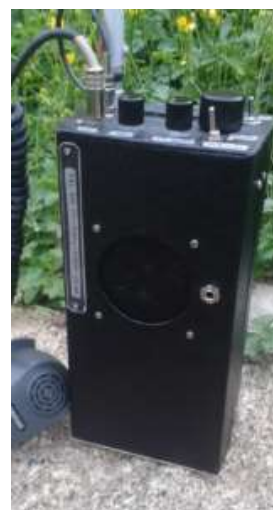
DK7IH SSB portable QRP transceiver (aka “Walkie Talkie”)
