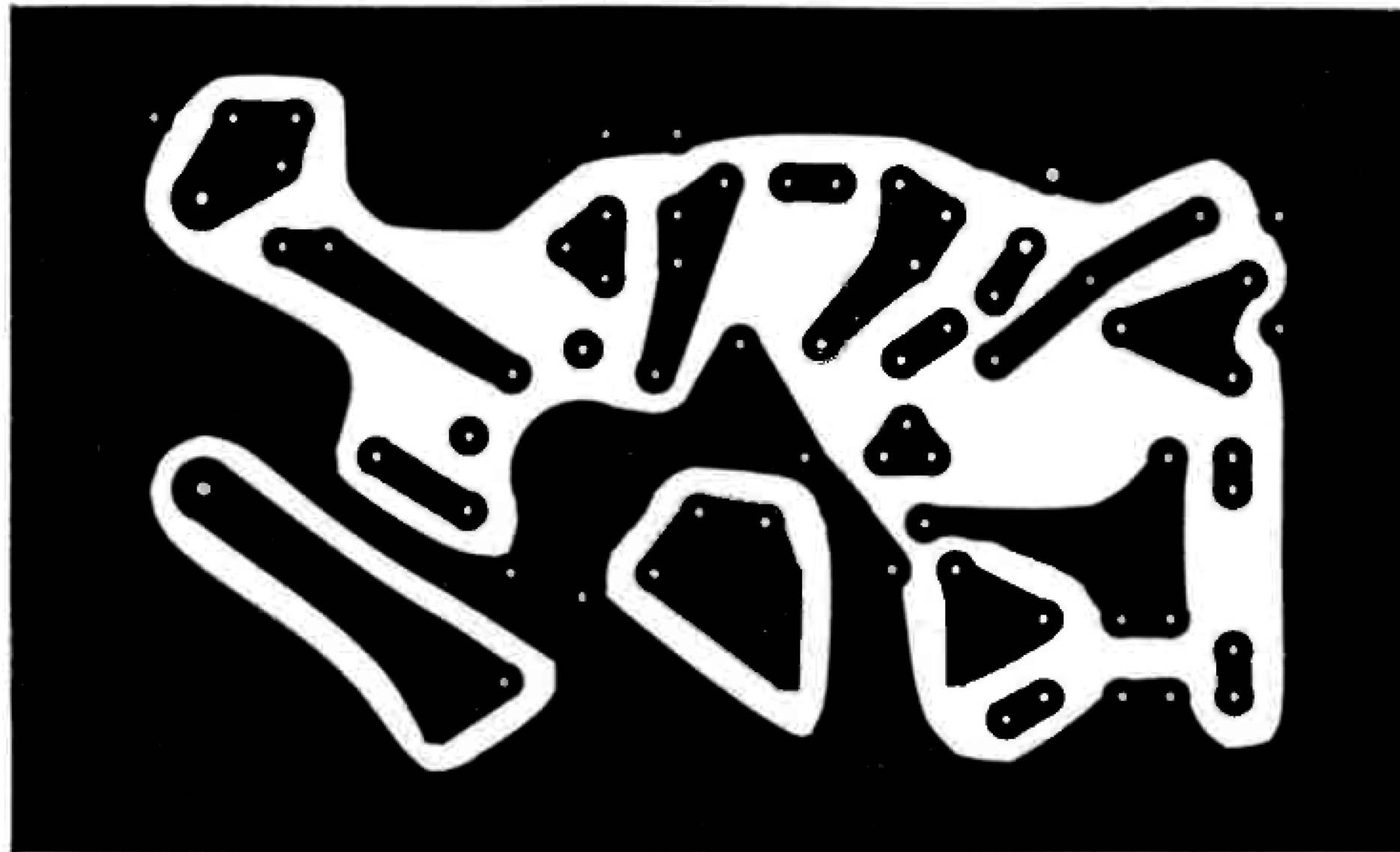
Actual-size photo shows foil side of printed circuit board (top); component side of board is at right. Observe polarity markings when installing diodes and electrolytic capacitors.
