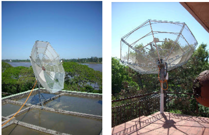
Figure 9 The identical 3.7 m antennas for the phased array: the W at left, the E at right.
